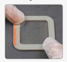
Robust & durable the new Elcometer 135C patches use a high quality adhesive, ensuring a water-tight seal during test.
