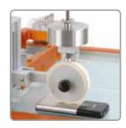
The rapid tool change system allows the user to test the samples in accordance with a wide range of National and International Standards on both flat and curved samples simultaneously.
