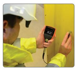
The gauges have all the features and functionality necessary to measure material thickness and velocity on virtually any material in a wide range of applications.
