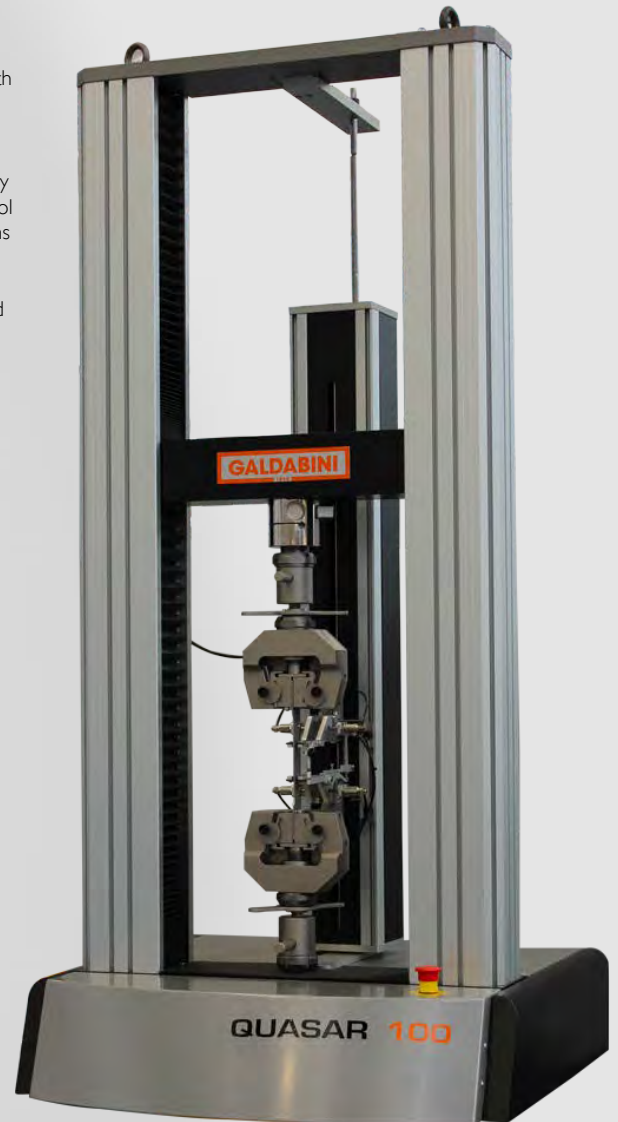
Universal testing machine Quasar 100 with manual wedge grip, Micron extensometer
