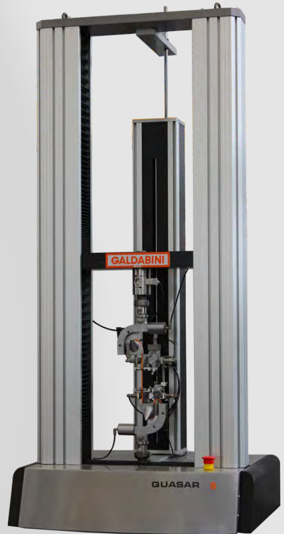
Universal testing machine Quasar 5 with Micron extensometer
