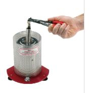
Extracting Tool enables the sample chamber to be handled easily and safely.
