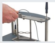
Detail of the PT100 probe holder drip tray for specimen holder, complete with handle
