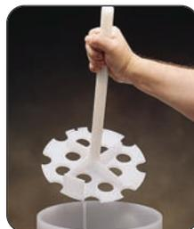
The polyethylene sample splitter consists of a thick walled cylindrical vessel with a disc churn. A center handle extends through the cover and a locating notch keeps it oriented in one direction. A small polypropylene spring-loaded spigot drains the subsamples into bottles for delivery to the water quality laboratory. A carrying handle makes carrying the full or empty vessel easy. Lid and spigot are replaceable.
