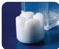
**Cell** magnetic stirring bars are designed specifically for use with spectrophotometer cells, cuvettes or test tubes. The cell stirrer fits into standard 10mm spectral cells and provides rapid vertical and horizontal mixing with a minimum of vortexing when placed on a magnetic stirring machine. Centrifugal pumping action, generated by the cross channels in the upper face, mixes without aeration. Page 388.
