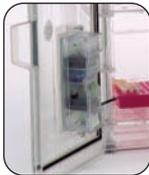
Door can be secured with tamper-evident tags or padlock
