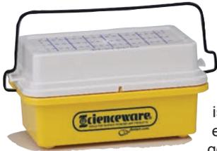
This cooler safely holds thirty-two 0.5, 1.5 or 2.0ml microcentrifuge tubes or cryogenic vials at a temperature below -15°C for approximately 1½ hours. The polycarbonate cooler body is filled with a non-toxic gel, which can not contact tubes, ensuring that markings and labels on tubes are safe. The gel-filled polycarbonate lid extends temperature holding time and is secured closed with a built-in wire carrying handle.
