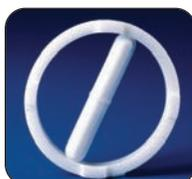
**Spinring®** stirring bars provide maximum stabilization of the magnetic stirring bar with the addition of a “hoop” around a standard octagonal bar. The friction fit of the “hoop” and bar allows them to spin as a unit. By presenting a greater surface area and wider profile, “spin out” is virtually eliminated. This particular arrangement is best suited for larger open-neck vessels, such as buckets and beakers. Page 382.
