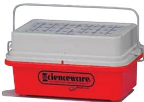
Benchtop sized cooler holds thirty-two 0.5 or 1.5ml microcentrifuge tubes at a temperature below 0°C for approximately 3 hours. The polycarbonate cooler body is filled with a non-toxic gel, which cannot contact tubes, ensuring that markings and labels on tubes are safe. The gel-filled white polycarbonate lid extends temperature holding time and is secured
