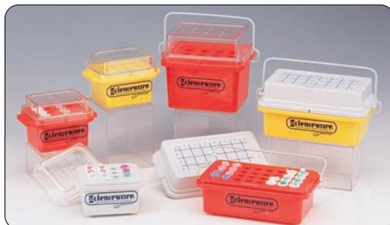
*“Hold the Cold” without a Mess! Use in transit and on the bench, cooler walls are filled with a non-toxic gel that does not come in contact with contents of cooler.*
