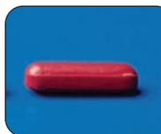
**Micro (Flea)** magnetic stirring bars are designed for stirring small volumes in vessels such as vials, tubes and gradient makers. Available in a variety of colors and sizes, micro (flea) stirring bars are particularly useful for environmental testing and life science applications in which small sample volumes need to be prepared and evaluated. Page 384-385.
