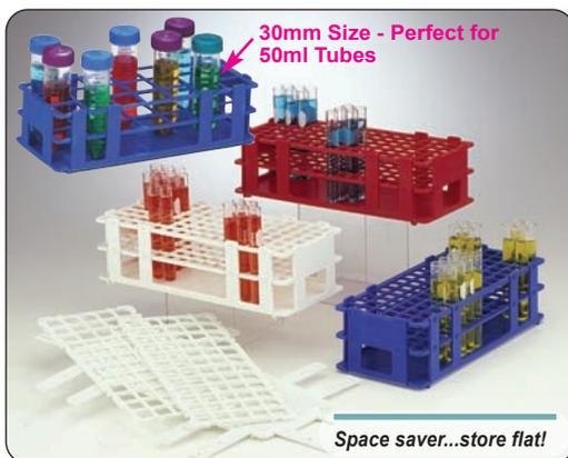
Each rack features end plates for labeling as well as numbered and lettered rows for tube identification. Interlocking feet allow stacking of racks for storage. Dimensions for all racks are 24.6 x 10.4 x 6.4cm high (9.7 x 4.1 x 2.5") and they assemble in seconds. Steam autoclavable at 121°C (250°F). **Per each, 8 per case.**
