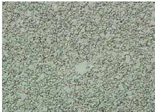
Tungsten-Carbide, etched with HNO3 (2000X - DIC)
