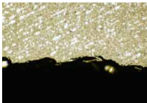
Silicon edge damage after sectioning with medium grit diamond wafering blade.
