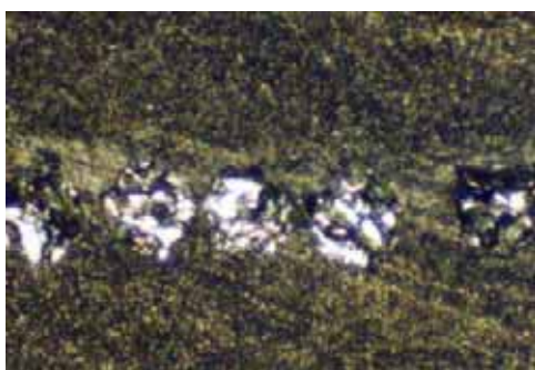
Boron-graphite composite sectioned with medium grit diamond wafering blade. Boron fibers damaged.
