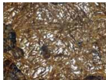
1095 Steel, Water Quenched (1000X), 2% Nital etchant - Martensite structure
