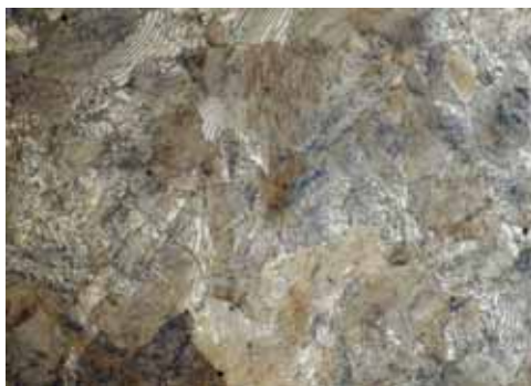
1095 Steel, Furnace Cooled (400X), 2% Nital etchant - Pearlite structure
