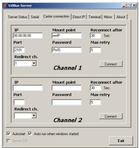
This tab allow to make a connection to one or two Ntrip Caster. Specifically, any client will connect to a Caster that also known of correction distributor.
