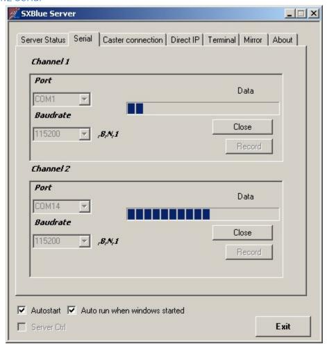
This tab is to make the setting of two port depending on the baud rate and the com port of your SXBlue receiver. That's a possibility to generate different type of corrections via theses port with only one SXBlue receiver or two SXBlue receivers. Any port can handle correction such as RTCM 1/3/9, CMR, ROX, etc. The scroll bars allow you to view the activity of the port.
