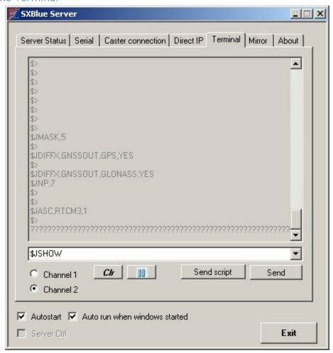
This tab allow to view the NMEA Message coming out from both channel 1 & 2 or to send configuration commands to the receiver. The "CLR" button to clear the terminal view. The "Send Script" button to send a configuration script to the SXBlue receiver.
