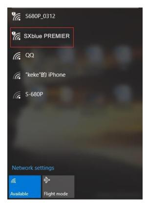
For example, search the WIFI hotspot broadcasted by a SXBLUE PREMIER receiver using laptop PC, choose the WIFI hotspot and click on connect button to establish the connection without password.
