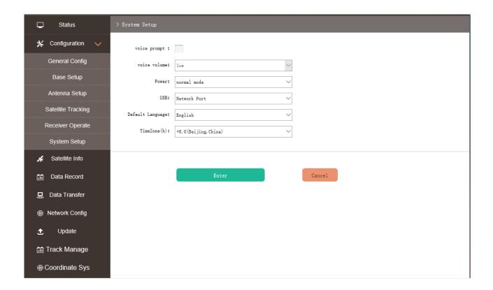
**USB** scroll down list present two option. If you want to download/transfer RAW data with USB cable (recommended), **USB** mode needs to be selected. The internal memory of the SXBLUE PREMIER will be accessible such as external device when the receiver is connect with computer via USB cable.
