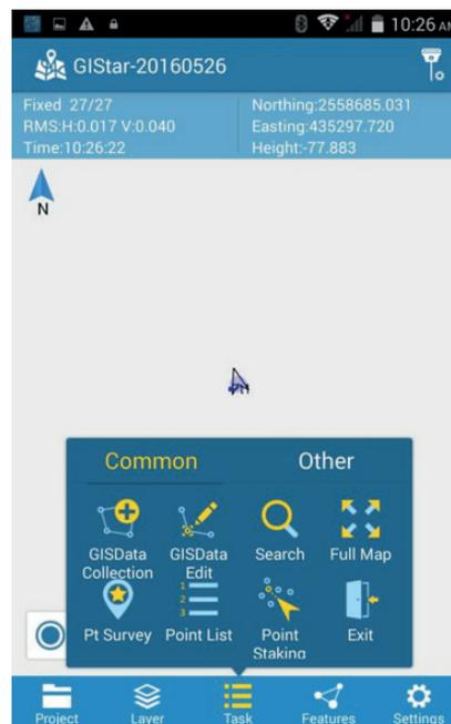
10) make sure that the instrument is leveling on a point, and the coordinates are stable at this position, tap on button to collect the coordinates for this position.
