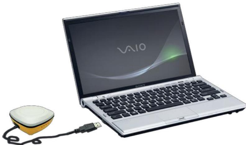
The micro USB port of SXBLUE PREMIER is default set as Ethernet function, then connect SXBLUE PREMIER receiver to computer via a micro USB cable. Run the IE explorer on computer and type IP 192.168.155.155 into IP address bar, then input the default username (admin) and password (admin) for login.
